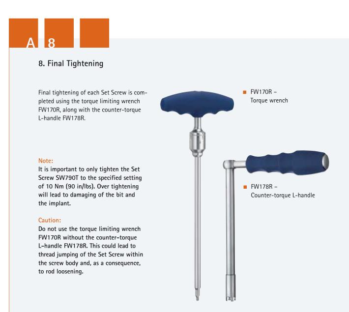
To properly tighten the Set Screw SW790T, the following steps should be performed:
